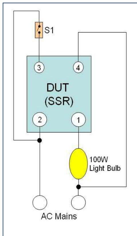
Fig 2; SSR bench test wiring diagram for an AC input / AC output SSR
